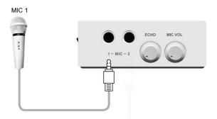
Adjust the microphone volume and echo level with MIC VOL and ECHO control knobs.
